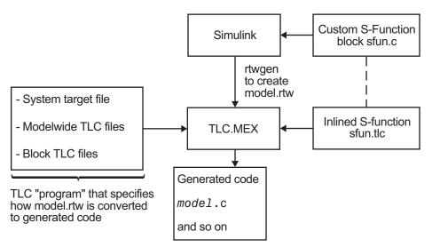
Just as a C program is a collection of ASCII files connected with #include statements and object files linked into one binary, a *TLC program* is a collection of ASCII files, also called *scripts*. Because TLC is an interpreted language, however, there are no object files. The single target file that calls (with the %include directive) all other target files needed for the program is called the *entry point*.
