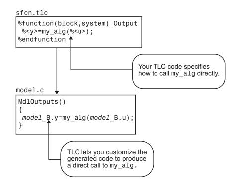
This is the inlining TLC file for a wrapper version of the timestwo block.
