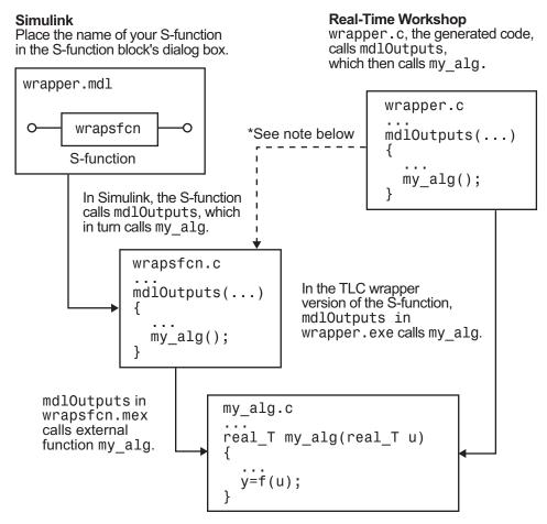
\*The dotted line is the path taken if the S-function does not have a TLC wrapper file. If there is no TLC wrapper file, the generated code calls mdl0utputs.
