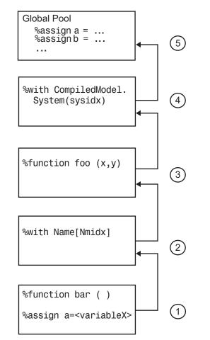
If a <code>%with</code> is included within a function, its associated scope is carried with any nested function call, as shown in the next figure.
