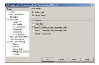
Selecting **Start TLC debugger when generating code** is equivalent to adding -dc to the **RTW System target file** field in the **Real-Time Workshop** pane of the Configuration Parameters dialog box. **4** Apply your changes and click **Build** to start code generation. This stops at the first line of executed TLC code, breaks into the TLC command-line debugger, and displays the following prompt:
